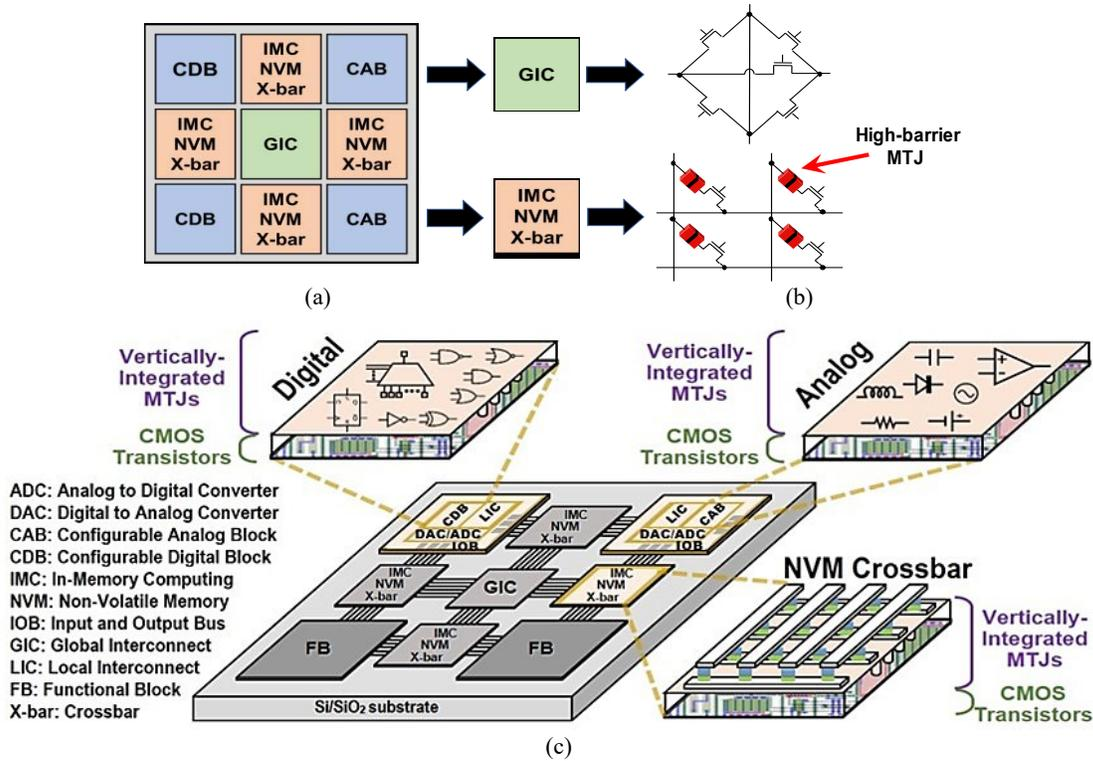
Fig. 1: (a) Single-Slice organization for proposed M-FPAA architecture, (b) M-FPAA routing and switch interconnect design, and (c) Hybrid Spin/Charge device realization as configurable blocks within the M-FPAA fabric.
