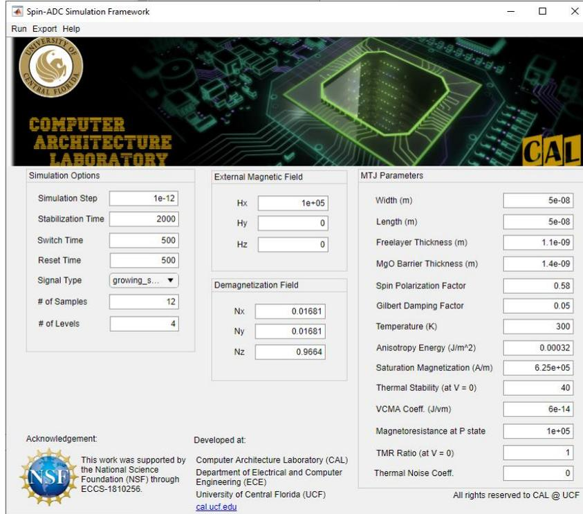
Figure 4: Spin-based ADC Interactive Simulation GUI.
