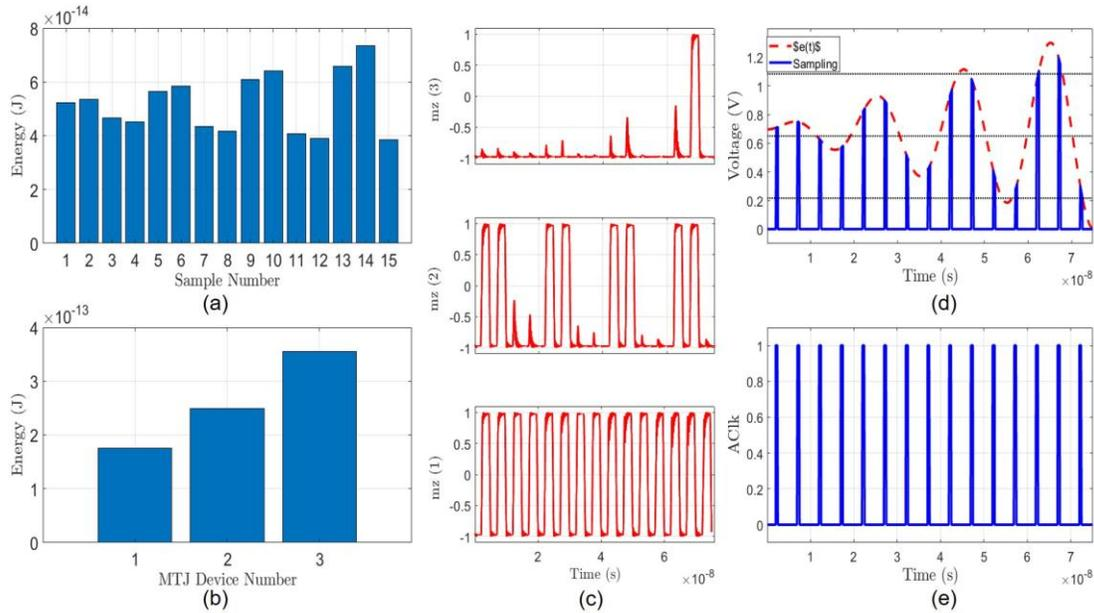
Figure 5: Simulation Run #1 using Input Signal= Growing Sinusoidal, SR=15 Samples, and QR=2 Bits.
