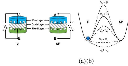
Figure 1: (a) VCMA-MTJ Structure, and (b) Energy barrier modification using VCMA Effect [1].
