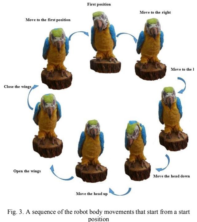
Fig. 3. A sequence of the robot body movements that start from a start position
