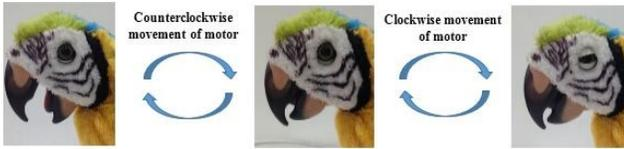
Fig. 4. Closing-opening the eyelids with clockwise movement of the head motor (right) - Closing-opening the beak with counterclockwise movement of the head motor (left)
