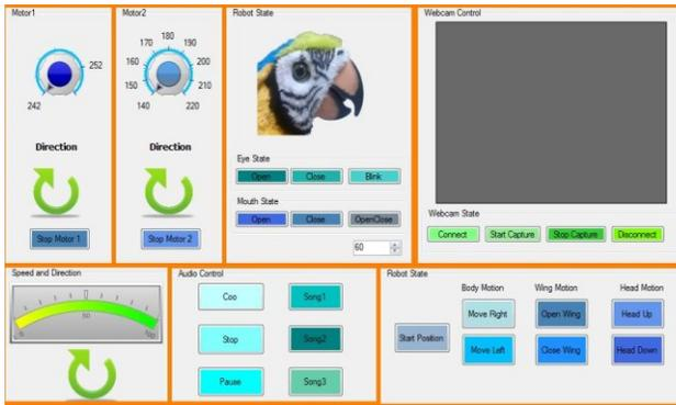
Fig. 8. The RoboParrot User Interface. The top-left boxes are the control for the body and head motors. The top-middle box, with the parrot head, shows the states of the robot's eye and beak. The top-right box is the camera view. The bottom-left gauge shows the sounds level. The bottom-middle box are different songs that can be played for a child. The bottom-right box are specific controls that the operator can select such as moving left or right and opening-closing wings
